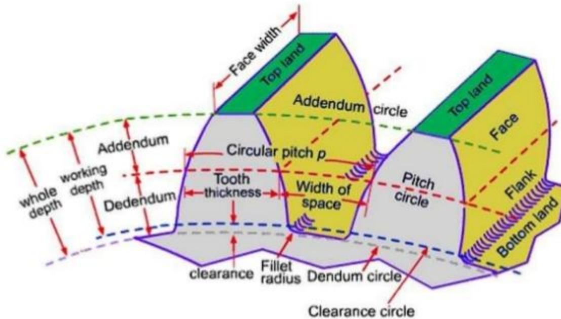
**16. Tooth thickness.** It is the width of the tooth measured along the pitch circle.
