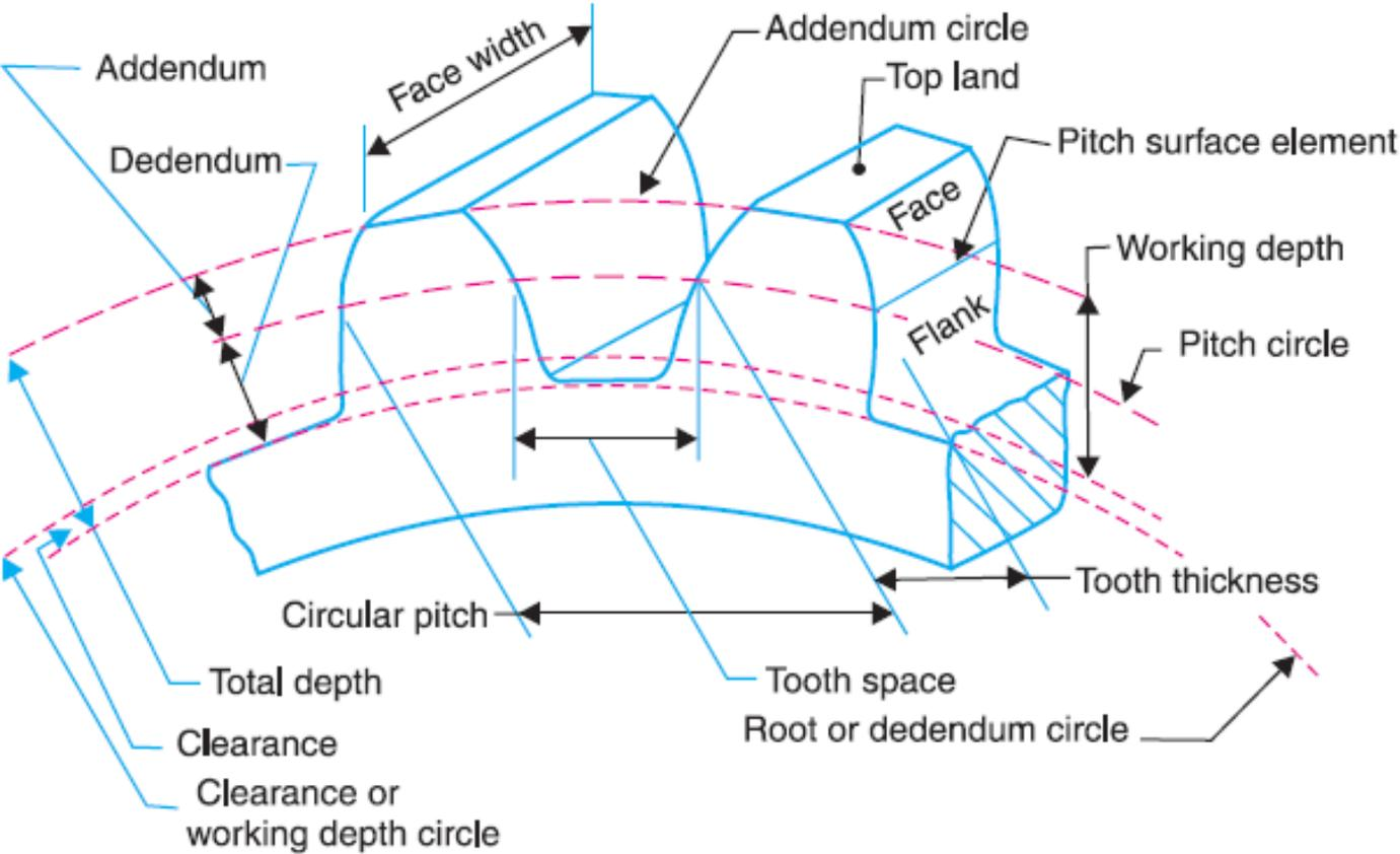
**Fig. 12.5.** Terms used in gears.
