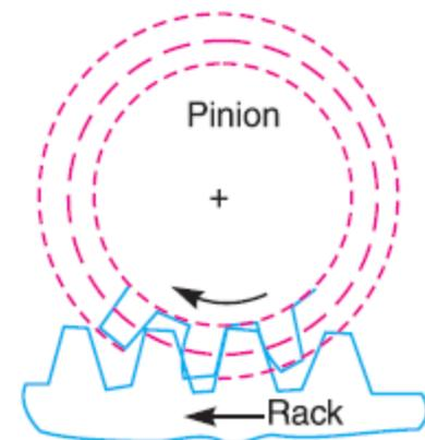
Fig. 12.4. Rack and pinion.
