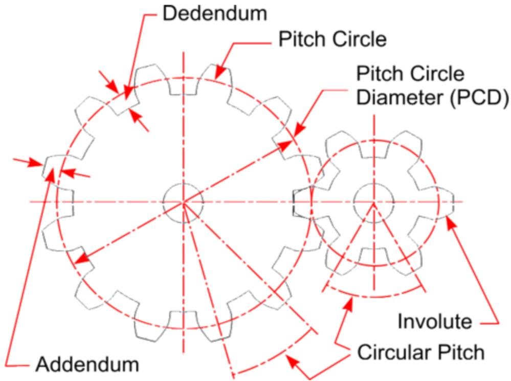
**1. Pitch circle.** It is an imaginary circle which by pure rolling action, would give the same motion as the actual gear.
