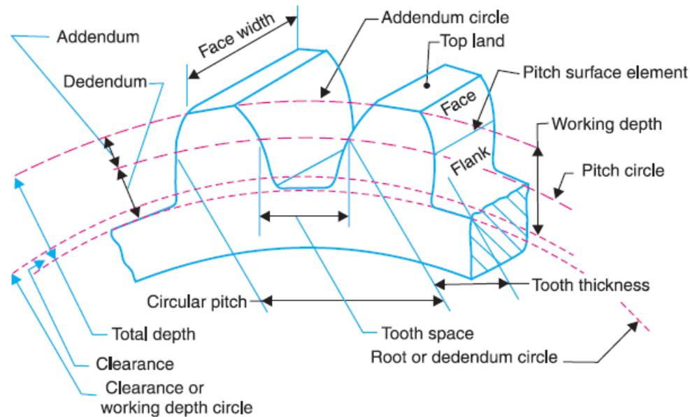
Fig. 12.5. Terms used in gears.
