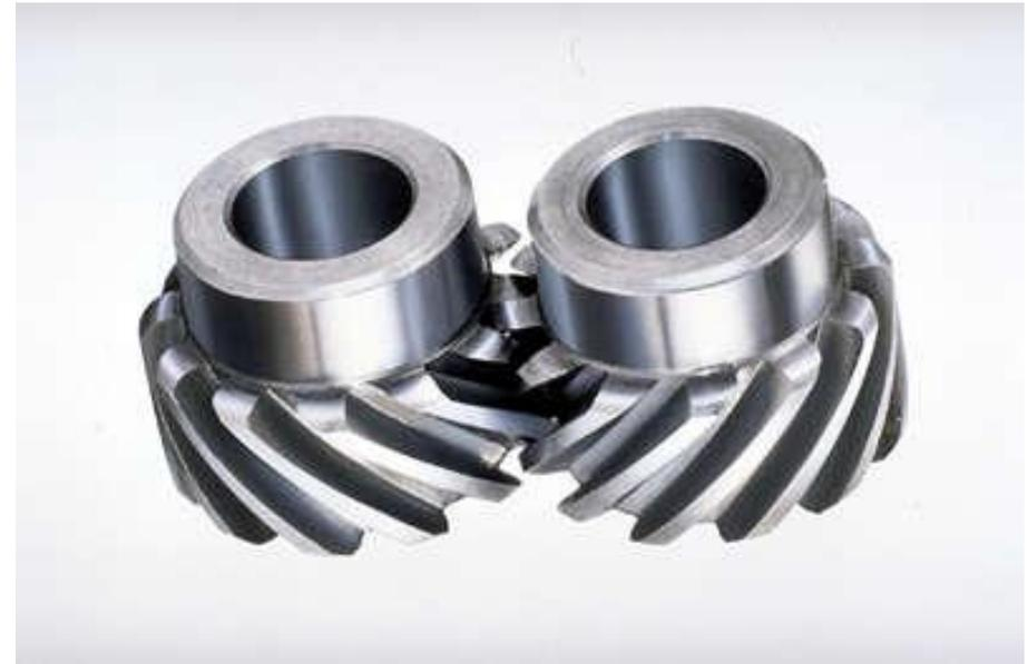
**Bevel Gears:-** The gears used to transmit motion from one shaft to another when their axes intersect are called **“BEVEL GEARS”** and the arrangement is called Bevel Gearing. The bevel gears, like spur gears, may also have their teeth inclined to the face of the bevel, in which case they are known *as helical bevel gears*.
