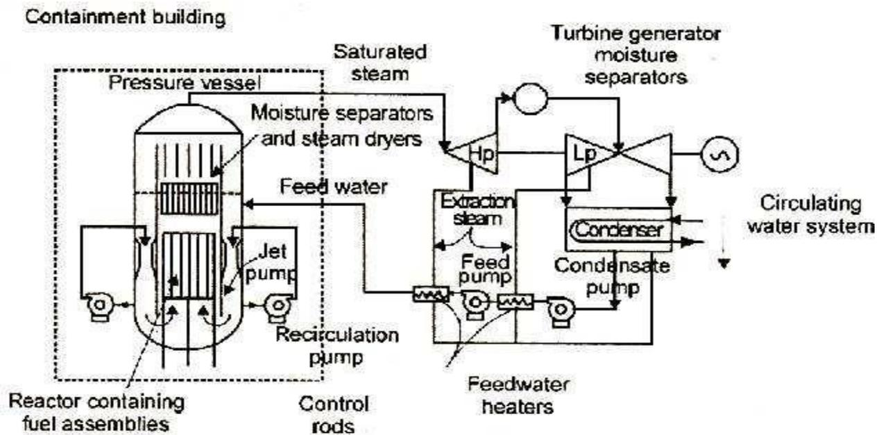
**Figure: Schematic for a boiling water reactor.(BWR)**
