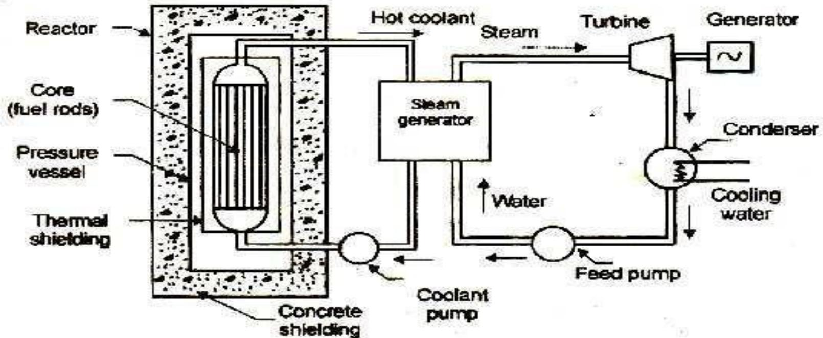
Figure : Nuclear Power Plant layout
