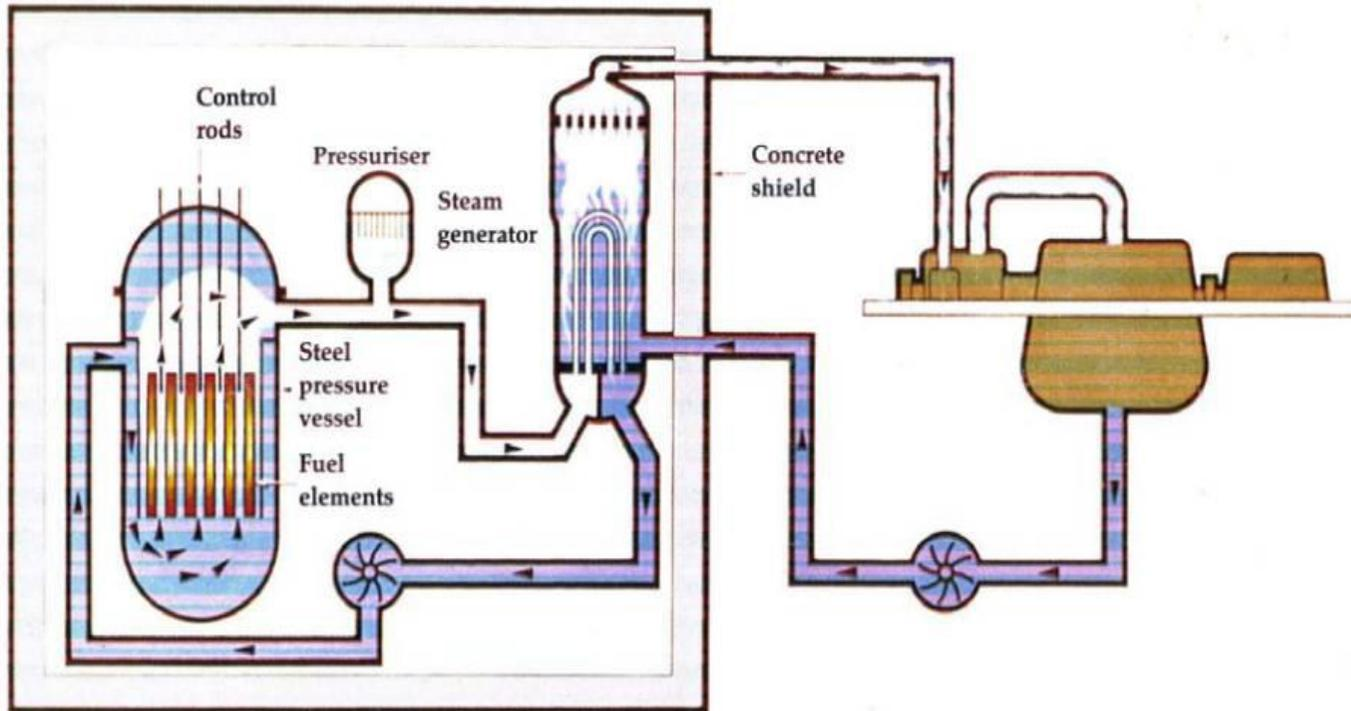
**Pressurized Water Reactor (PWR)**
